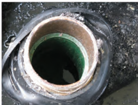
Figure 43 Tank 1 fill point opening — no melting of green plastic pipe
