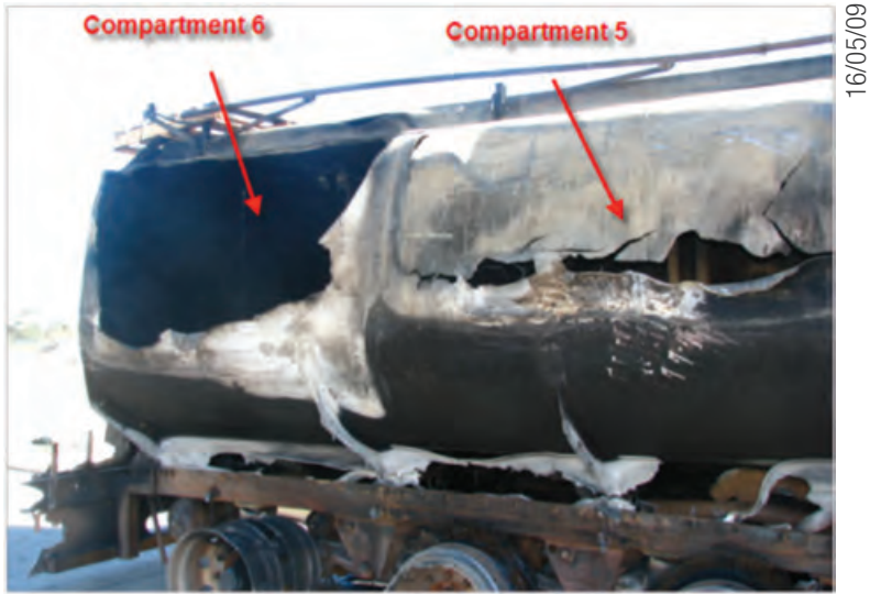
Figure 28 Ruptured compartments on the rear driver side of the fuel tanker
