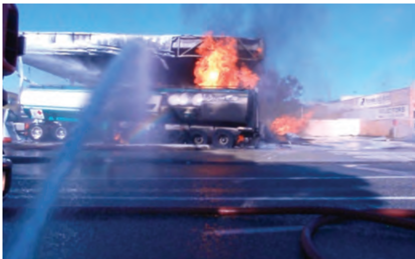
Figure 16 Fire on top of compartments 5 and 6, and burning LP Gas cylinders in cage in the background [photograph courtesy of FESA]
