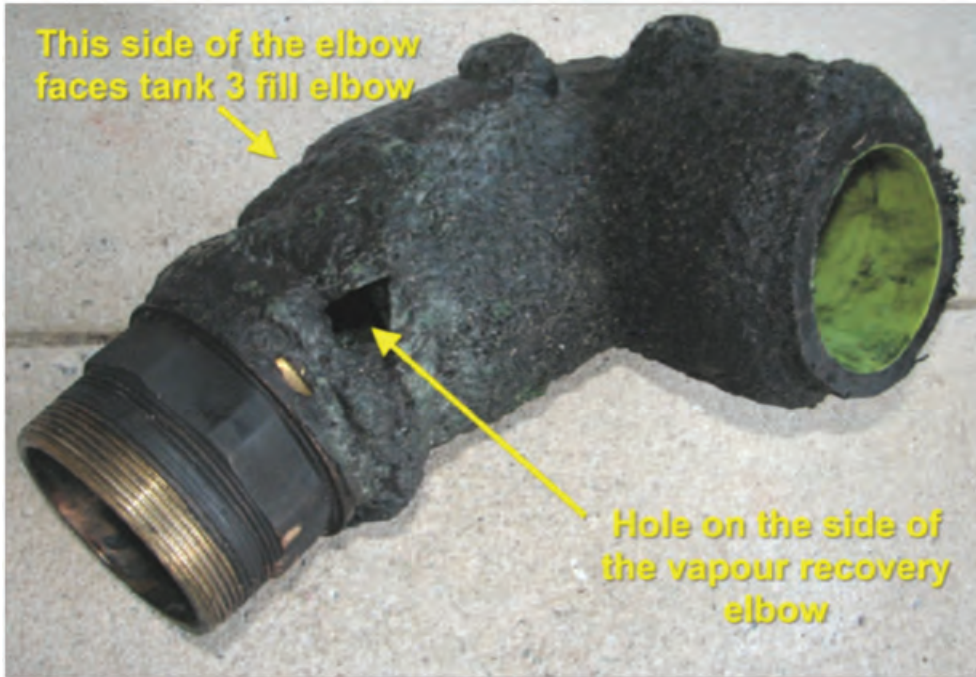
Figure 39 Hole in vapour recovery elbow pipe and location relative to tank 3
