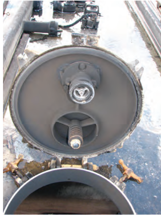
Figure 36 Inside surface of manhole cover with pressure-vacuum vent (top) and emergency vent (bottom)
