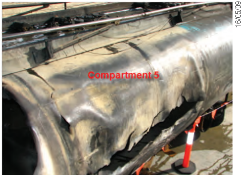
Figure 29 Side view of the ruptured section of compartment 5
