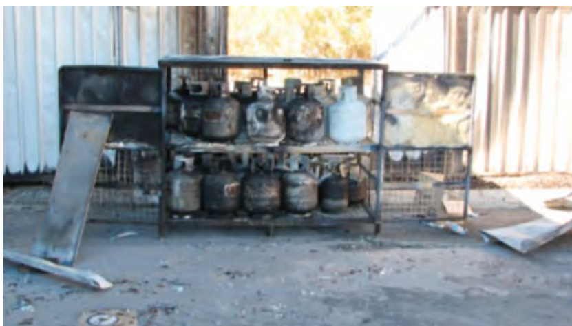
Figure 26 Fire-damaged LP Gas exchange cylinder cage
