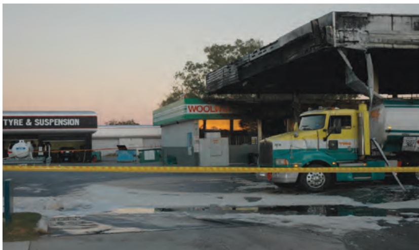
Figure 18 Tanker vehicle after the fire was extinguished. The aboveground bulk LP Gas tank is visible on the left of the photograph [photograph courtesy of FESA]
