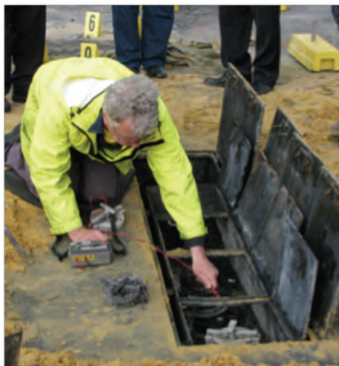
Figure 56 Measuring electrical conductivity at the service station after the fire
