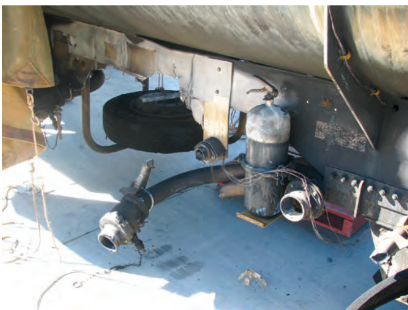
Figure 27 Damaged fire extinguisher beside the vapour recovery point, and one outlet valve still attached to the product line
