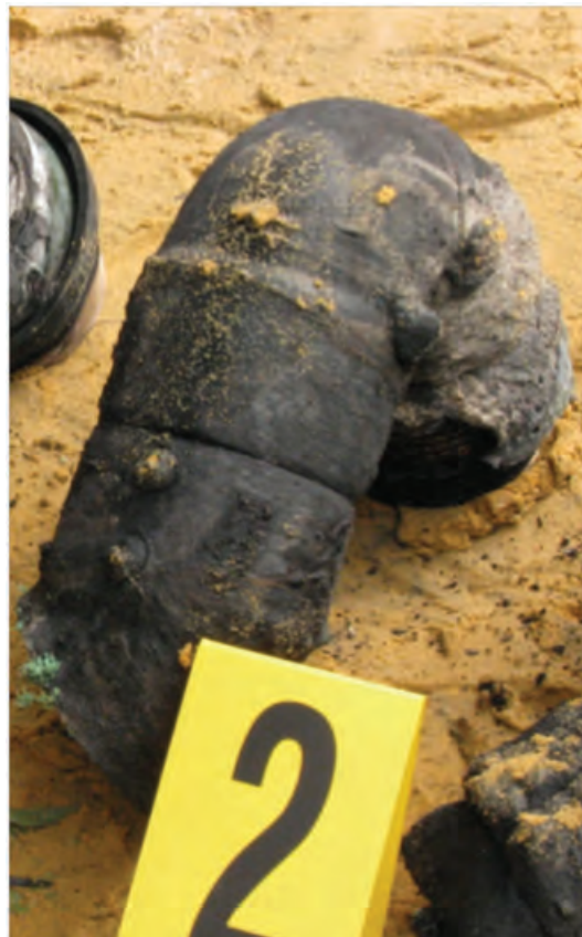
Figure 48 Fill pipe elbow of tank 2 — pipe is fire affected
