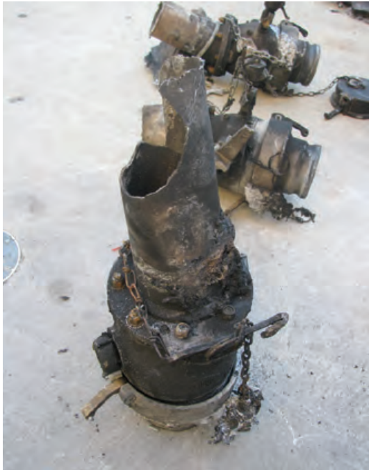
Figure 32 Detached tanker outlet valves
