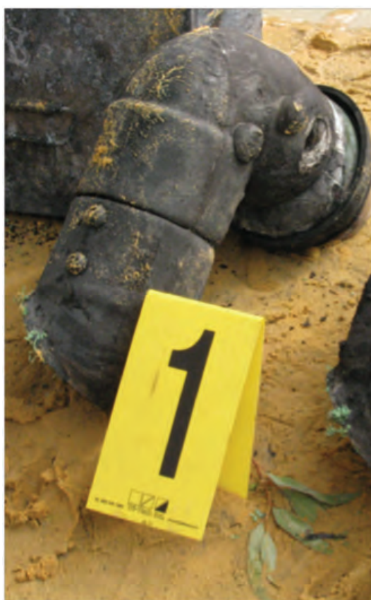
Figure 45 Fill pipe elbow of tank 1 — pipe is not significantly fire affected
