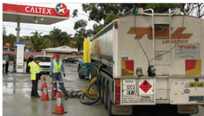
Figure 57 Typical arrangement for a tanker delivering fuel into underground tanks at a service station
