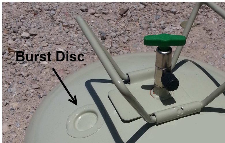
Figure 1 Examples of non-refillable gas cylinders fitted with burst disc.
