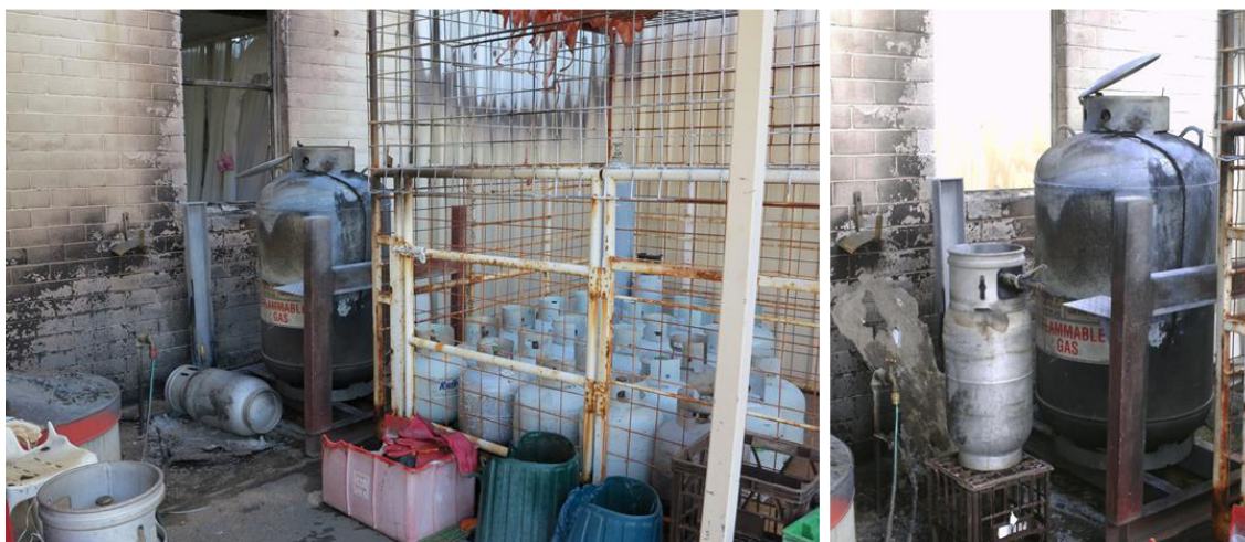
Left: The incident scene. Right: Re-creation of the cylinder setup used for decanting.
