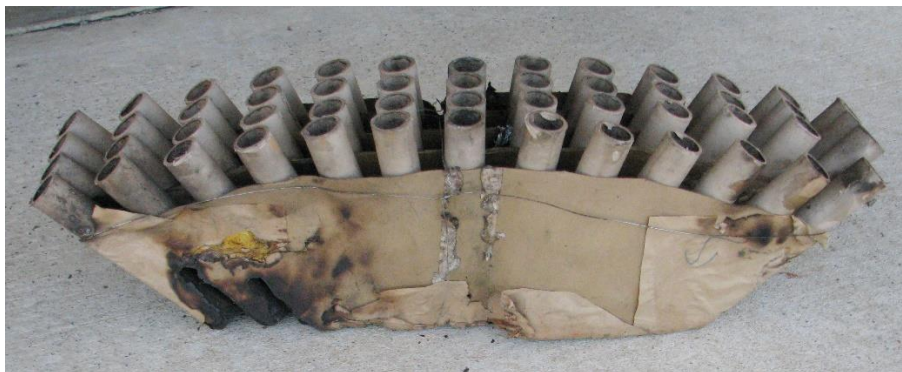
The spent 29 mm 52-shot fan firework involved in the incident. The burn mark is unrelated to the incident and there was no evidence of malfunction.
